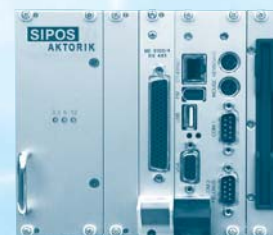
Actuator control system SIMA Master station
