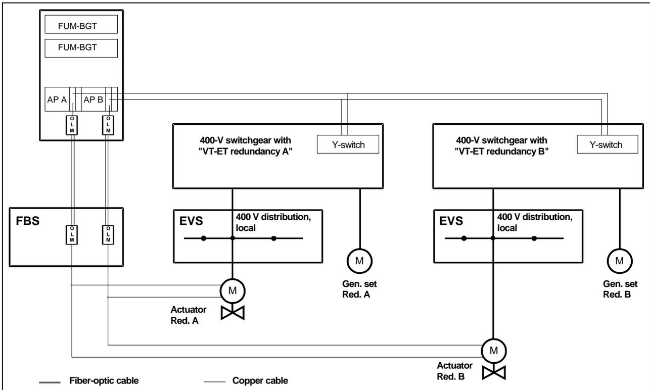
**Fig. 2** Redundancy Concept
