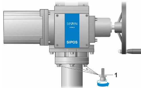
Fig. 1: Mounting actuator to linear thrust unit
