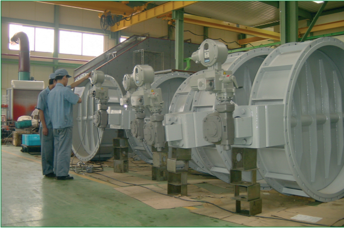
Fig. 5: DN 1800, PN 1.6 butterfly valves with variable speed actuator for control of air feed in a steel plant furnace
