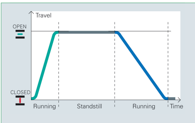
Fig. 6: Different speeds for OPEN/CLOSE direction can be selected and programmed from seven available speeds
