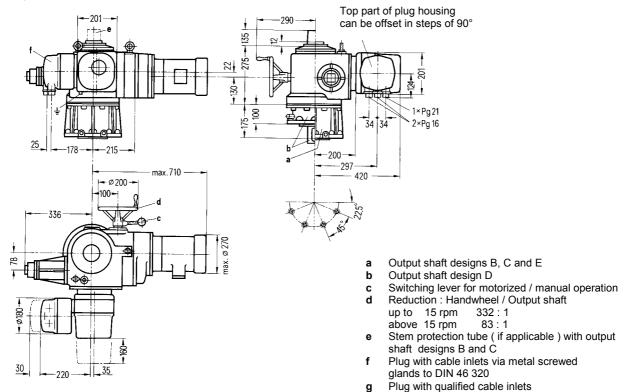
Rotary actuator M76371 – S, S – SIWI – AS series
