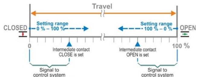
Fig.: Intermediate contact function principle
