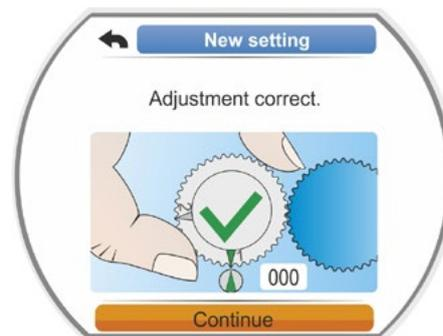
Fig. 9: First end position setting is correct
