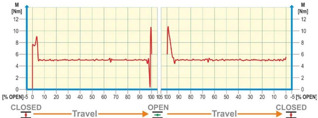
Fig.: Example of a valve torque curve
