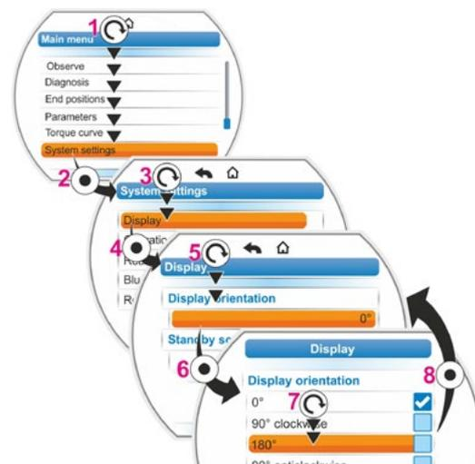
Fig. 2: Change display orientation
