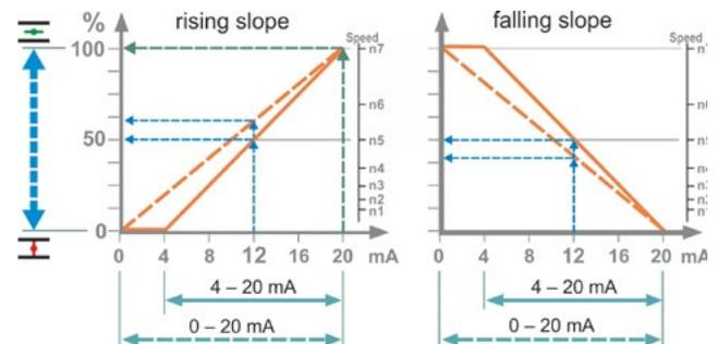
Fig. 2: Conversion 0/4 – 20 mA to 0 – 100 % or to speed with different curve
