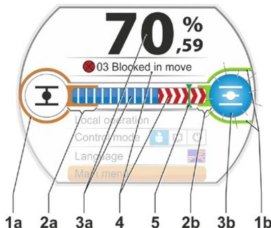
Fig. 1: End position symbols and progress bar
