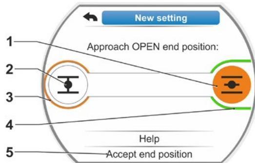
**Fig. 4: Approach end position in OPEN direction**
