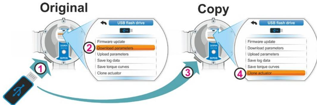
Fig. 1: Clone actuator procedure
