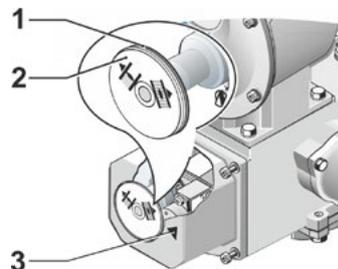
**Fig. 2: Adjust position indicator**
