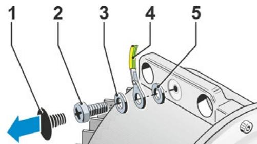
**Fig.: Fit potential conductor**
