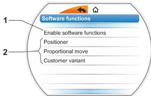
Fig. 1: Indication in the display: 'Software functions' menu
