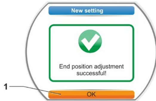
Fig. 8: End position setting complete
