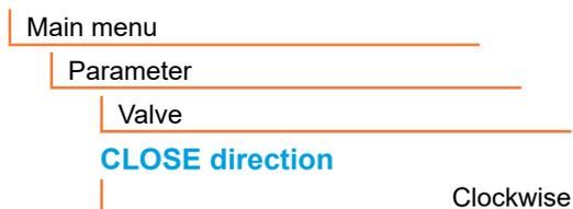
Fig. 1: Navigation to ‘CLOSE direction’ parameter
