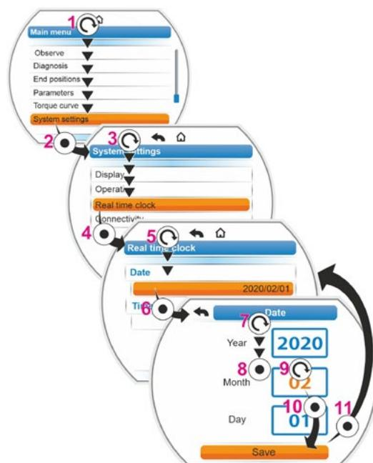
Fig.: Adjust real time clock
