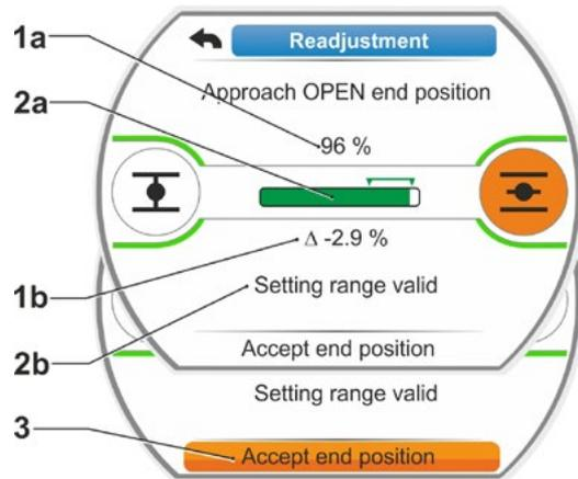
Fig. 4: Accept new end position
