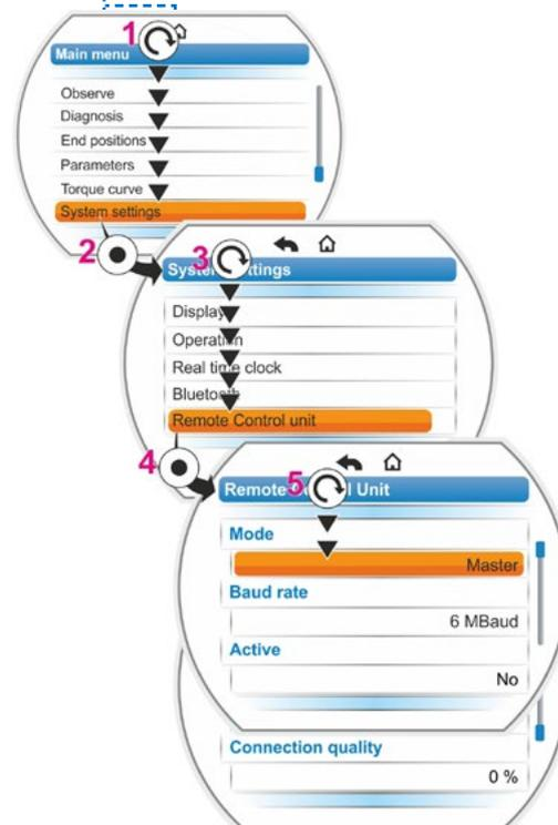
Fig. 3: Activate remote control unit
