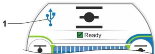
Fig. 2: Indication in the display: Communication via USB
