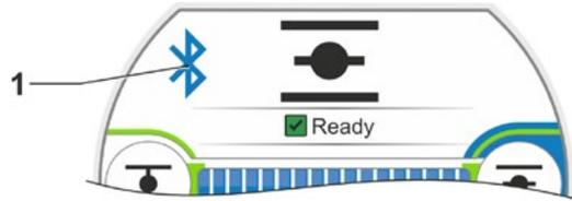
Fig.: Indication in the display: Communication via Bluetooth
