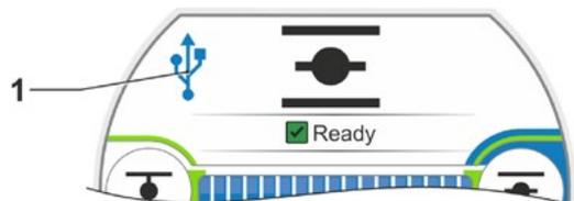
Fig.: Indication in the display: Communication via USB
