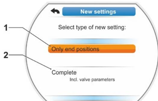
Fig. 2: End position setting with or without parameters
