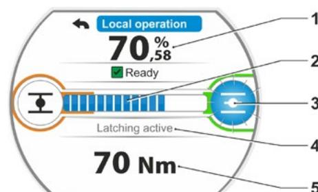
Fig. 4: Indication during operation
