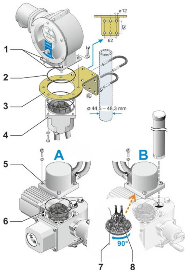
**Fig.: Separate mounting**
