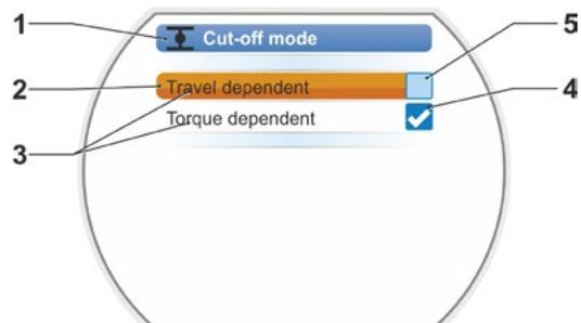
Fig.: Cut-off mode end position CLOSED menu
