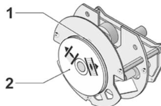
**Fig. 3: Position indicator for 2SG7**
