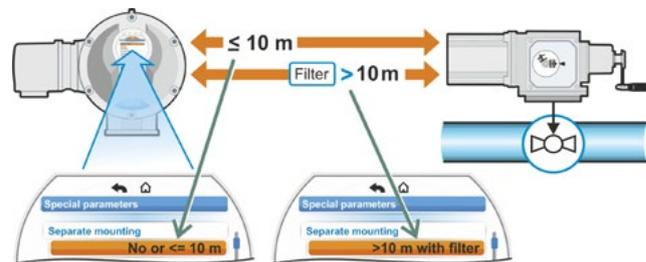
Fig.: Separate mounting
