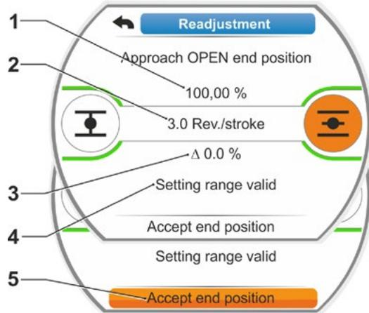
Fig. 3: Approach and accept new end position
