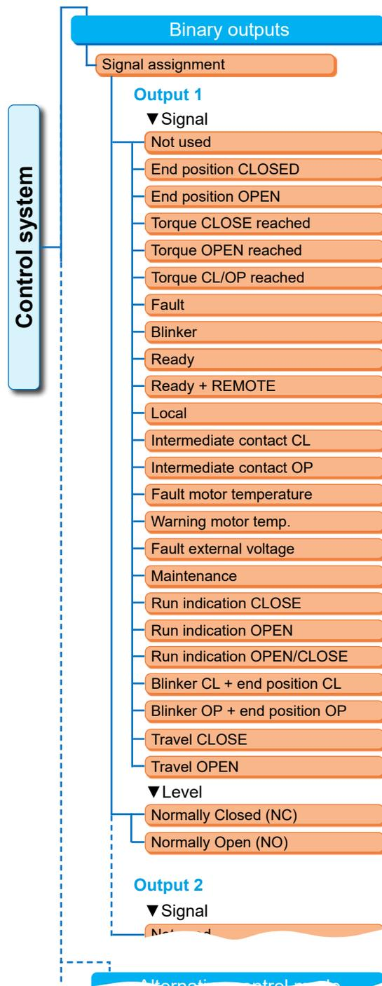
Fig.: "Binary outputs" menu parameters
