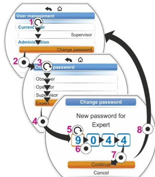
Fig. 2: Assign user access level
