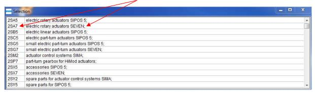
After the selection, the selection window closes and will open again after 2.5 seconds reserved for checks and calculations (may be changed in the "StanUni.ini" configuration settings file) for the next selection(s).
